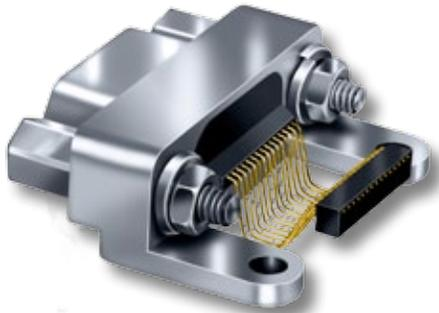
**Surface Mount Micro-D** – These connectors feature .025 inch terminal spacing and an alignment strip for accurate registration. The integral mounting legs provide a ground path.
