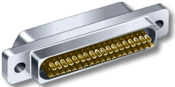
**Micro-D Solder Cup Termination**—These connectors feature gold-plated TwistPin contacts for best performance. Use with #26 or smaller stranded or solid wire. Specify nickel-plated shells or cadmium plated shells for best availability.
