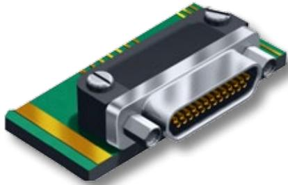
**Save Space On Your Circuit Board** – These Micro-D connectors feature .075 X .075 inch terminal spacing. Glenair's GMR7590 offers size and weight savings compared to traditional .100" pitch connectors.
