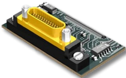
**High Performance** — These connectors feature goldplated TwistPin contacts for best performance. PC tails are .020 inch diameter. Specify nickel-plated shells or cadmium plated shells for best availability.
