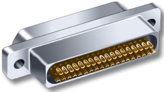
*Glenair's Filtered Solder Cup Micro-D's* provide EMI solutions in a miniaturized M83513 type connector. These connectors feature ceramic capacitor planar arrays and ferrite inductors. Solder cups accept #26 thru #30 AWG wire, or specify oversize contacts for #24 gage wire.
