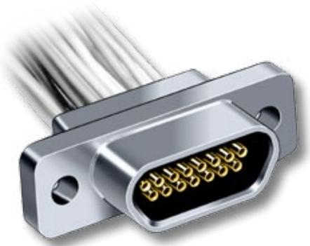
**Micro-D Pre-Wired Pigtails**—These connectors feature gold-plated TwistPin contacts and mil spec crimp termination. Specify nickel-plated shells or cadmium plated shells for best availability. 100% tested and backpotted, ready for use.
