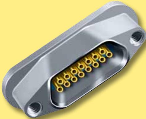
**Glenair's Hermetic Micro-D Connectors** feature fused glass insulators to provide an airtight seal. These connectors are 100% tested to meet a maximum leak rate of  $1 \times 10^{-8}$  cc's per second of helium.
