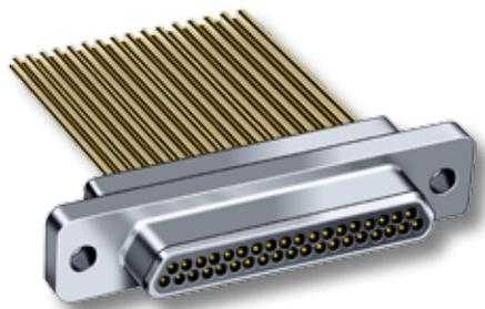
**Micro-D Uninsulated Pigtails**—These connectors feature gold-plated TwistPin contacts and mil spec crimp termination to gold-plated single strand copper wire. Suitable for soldering or splicing applications, the wire leads can be ordered either gold-plated or solder-dipped.
