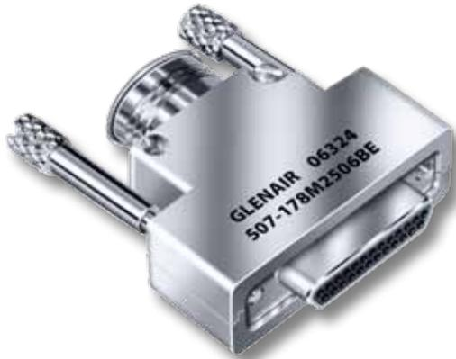
**Split Backshell With Elliptical Cable Entry** provides added room for larger wire bundles. Terminate cable shields with **BAND-IT®** microbands. This backshell features floating male screwlocks which allow full mating of the connector before the screws are fastened.
