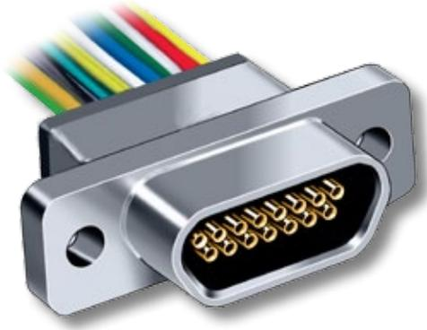
**Glenair's Filtered Pigtail Micro-D's** provide EMI solutions in a miniaturized M83513 Micro-D connector. These connectors feature ceramic capacitor planar arrays and ferrite inductors. Insulated wire is factory precision-crimped to TwistPin contacts for superior reliability in the most demanding environments.
