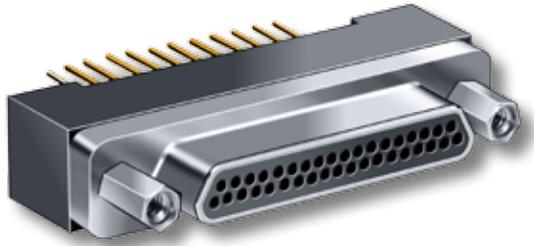
**Save Space On Your Circuit Board** – These Micro-D connectors feature .075 X .075 inch terminal spacing. Glennair's GMR7580 offers significant size and weight savings compared to traditional .100" pitch connectors.
