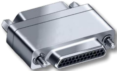
**Avoid Costly Redesign with Micro-D Filter Adapters.** Upgrade your existing cables and boxes to meet EMI requirements. These pin-socket adapters can be plugged into any standard M83513 connectors. Simply unplug your existing cable, install the filter adapter, and plug the cable into the adapter.
