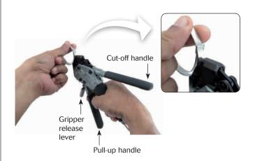
b ) Aligning the band and the tool with the shield termination area, squeeze the black pull-up handle repeatedly using short strokes until it locks against the tool body (this indicates that the band is compressed to the tool pre-calibrated tension).
