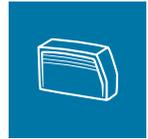
Connector housing for assembly on the cable. With expanded assembly space and side M50 cable entry.
