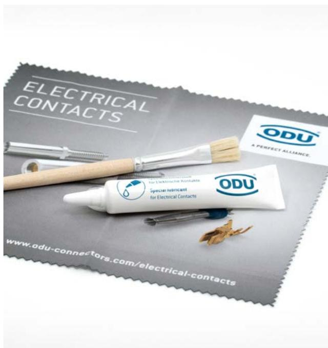
Contact lubrication improves the mechanical properties of contact systems. Cleaning the contact surfaces prior to lubrication is also recommended in order to remove pollution. With appropriate care, wear due to high mating frequency can be significantly minimised and the mating and unmating forces reduced. The cleaning and lubricating interval must be individually adapted to circumstances and should only be carried out with products recommended by the contact manufacturer.
