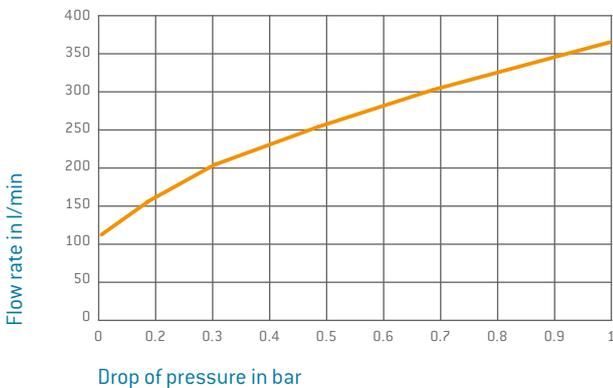
The flow diagram refers to the blocking variant with a maximum gap between socket and pin piece of ≤ 0.5 mm. The pressure reduction increases in the event of a changed gap measurement.
