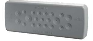
Using the latching clips, the **KES-GB** latches onto the outside of the housing wall. It is then screwed on from the inside, through the housing wall, using the integrated threaded bushes.
